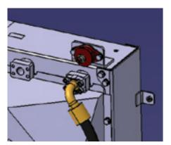
**Radiators Mounted on Rubber Mounts**
