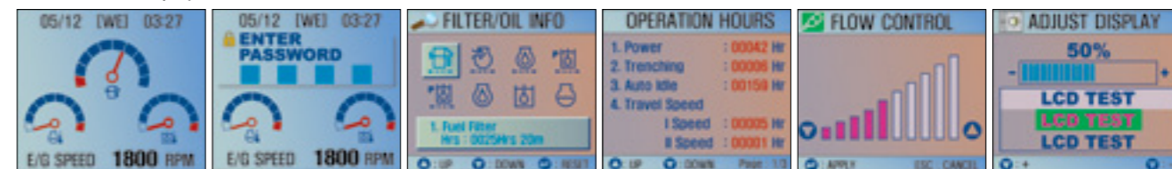
Standard screen Theft prevention function Filter/oil information Operation history Flow rate control Contrast control
