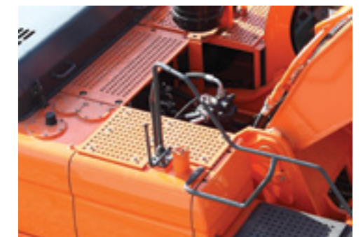
Cat walk (platform) as standard on DX420LCA Larger anti-slip surface on the upper structure for more safety.
