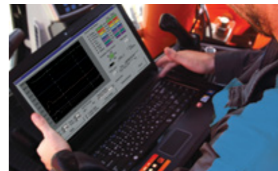
PC monitoring A PC monitoring function enables connection to the e-EPOS system. Thus, various parameters can be checked during maintenance, including pump pressures, engine rotation and engine speed. These can be stored and printed for analysis.
