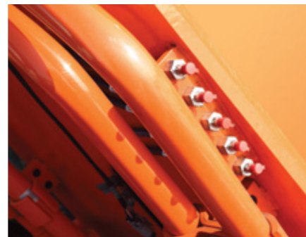
Remote greasing points To make maintenance easier, the arm and boom greasing points have been centralised. Remote & grouped greasing points on boom & arm.
