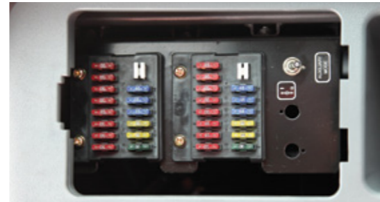
Convenient fuse box The fuse box is located in the storage compartment behind the seat, providing a clean environment and convenient access.
