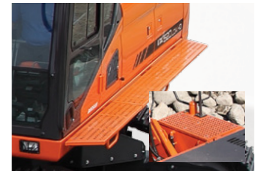
Cat walk (platform) as standard on DX480LCA-HD & DX520LCA-HD Larger anti-slip surface on the upper structure for more safety.
