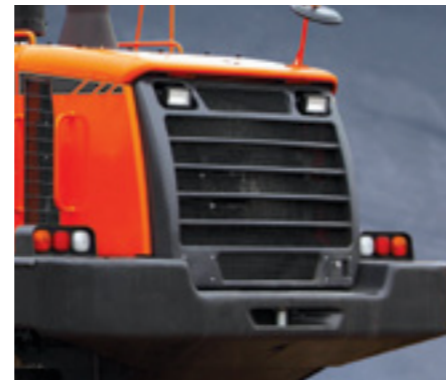
Radiator Grill (Steel structure)
